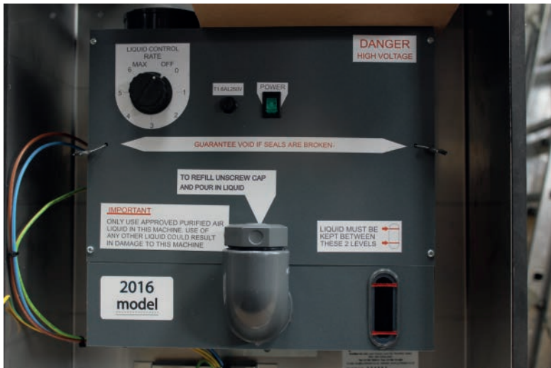
Figure 11 - Liquid Control Rate Knob and Filler Cap
